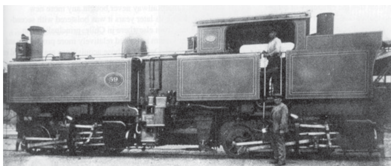
Kitson-Meyer no. 59 , with a Worthington feed water heater and therefore a divided tank. The bunker is also higher than on the earlier engines.
