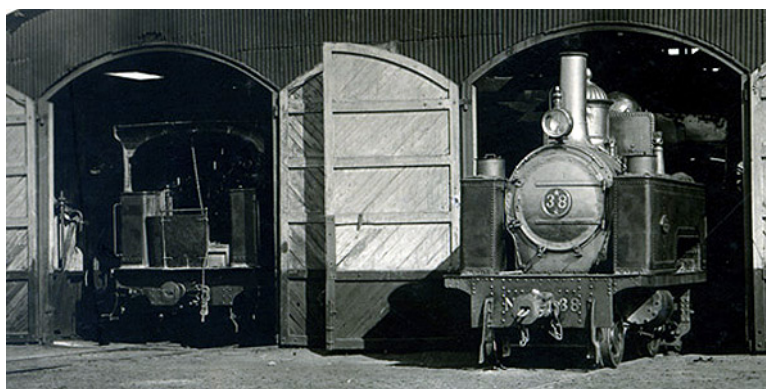
A pair of Sharp Stewart designed 'back-to-back' locos in Zapiga loco shed in 1929. On the right is 2-6-0T no. 38 , whilst the rear view of the engine on the left clearly shows the waist height screen that protected the crew from falls.
