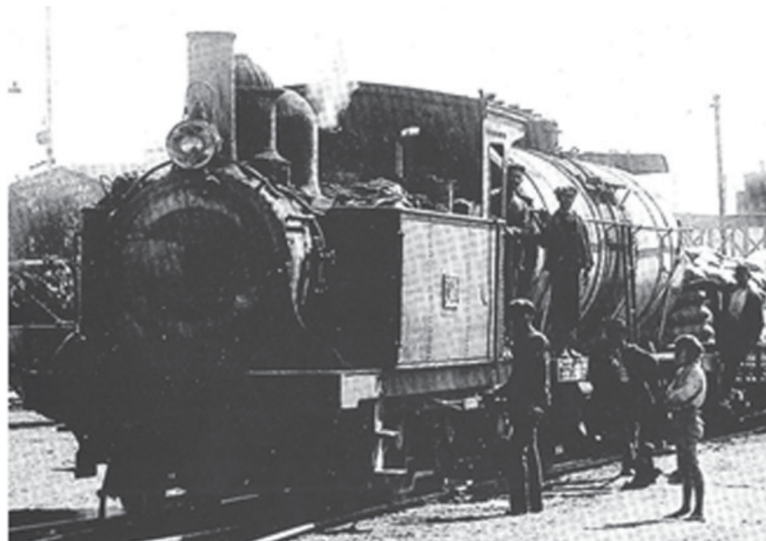
No. 24 somewhat later, with a different smokebox and chimney. The smokebox front panel now has a wide flare at the bottom in the same fashion as that on loco no. 25 .
