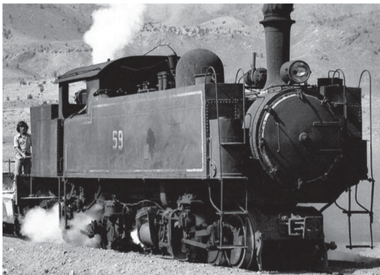
This shows no. 59 during its very last days as the railway was dismantled. Note the increased height of the much re-welded tanks and bunker. Photo found on a Chilean rail enthusiasts' Facebook page. Photographer unknown.
