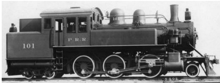
The Panama Railroad 100 series engines, as originally configured as 2-6-4Ts.
