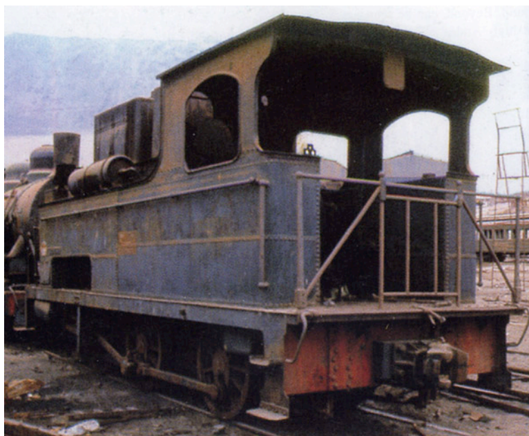
This rear view of. no. 70 by J. Hutzler in 1976, clearly shows the footplate extension and fixed railings that replaced the original narrow protective 'wall' at the back of the cab.
