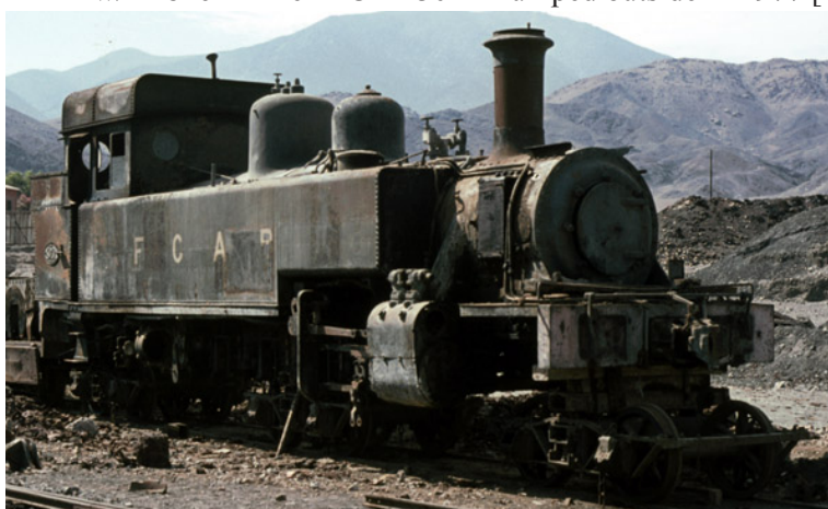
MCC's own photo of no. 30 , at Taltal in 1975, whilst supported on ambulance bogies during re-gauging work.
