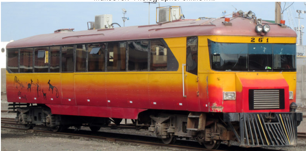
Railcar 261 in its present guise. Whilst the windows, paintwork and roof-mounted AC units suggest radical changes, it seems likely that the bogies, frame and basic body
