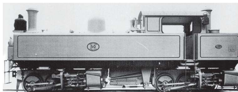
The first FC de Taltal Kitson-Meyer, no. 50, as illustrated in Kitson publicity material. Note that FC de Taltal Kitson-Meyers were built with enclosed cabs whilst those for the FCTT had more open cabs.
