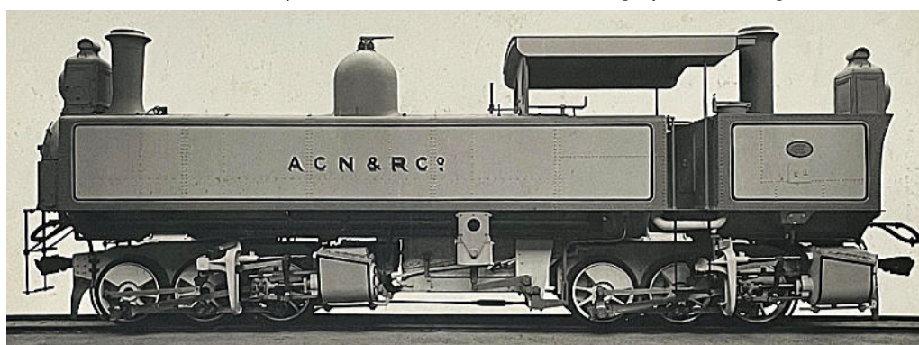
Kitson builders' photos, via Donald Binns' FCTT book. This one was probably no. 12 . Note the larger rear chimney on this 1895 loco.
