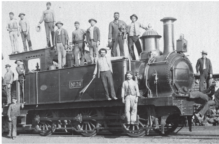
Photo kindly provided by Señor Pablo Moraga. The works plate in front of the cab doorway is definitely in Sharp Stewart's style, but there is also a Nitrate Railways painted ownership plate on the bunker side behind the cab.
